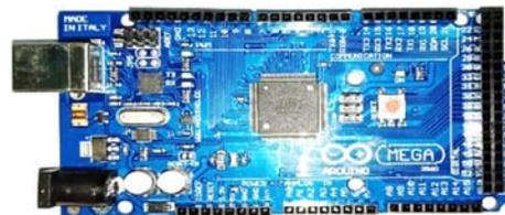
Gambar 2.2 Arduino Mega2560
